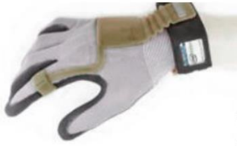
Figure 3. Gloves with integrated RFID reader (Mocan and Draghici, 2018)
