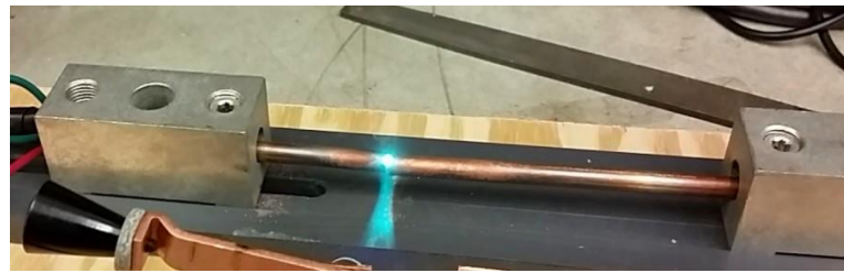
(a) A dc arc generator creates a dc arc.
