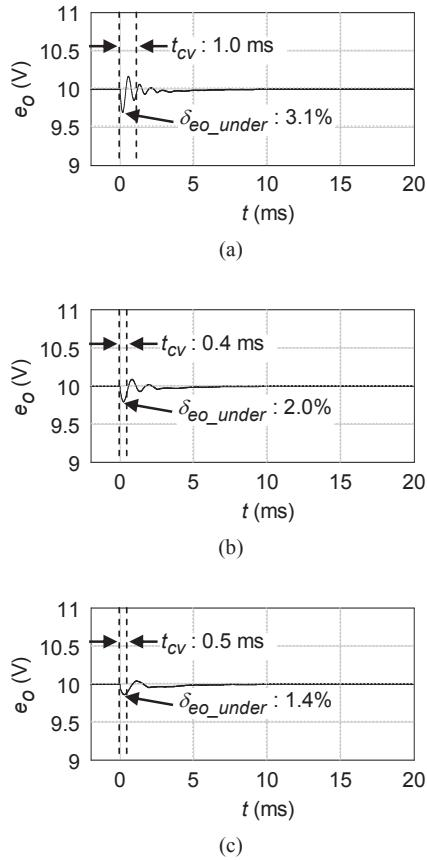
Fig. 6. Transient response of output voltage,  $e_o$ , when a number of switching periods between sampling points in PID control,  $M_{PID}$ , is 10: (a) output smoothing capacitor,  $C$ , is equal to  $200 \mu\text{F}$ , (b)  $C$  is  $400 \mu\text{F}$ , and (c)  $C$  is  $800 \mu\text{F}$ .
