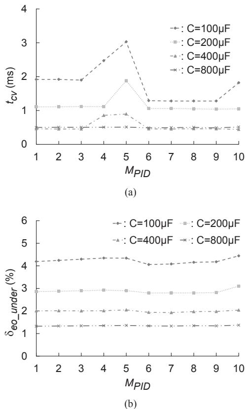
Fig. 4. Transient characteristics of output voltage,  $e_O$ , against a number of switching periods between sampling points in PID control,  $MPID$ : (a) convergence time of  $e_O$  within plus-minus 1% of reference voltage,  $t_{cv}$ , (b) undershoot of  $e_O$ ,  $\delta_{eo\_under}$ .
