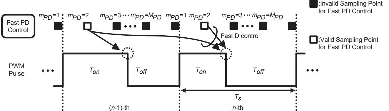
Fig. 3. Timing chart of fast PD control.
