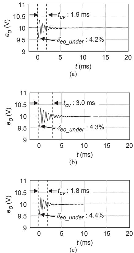
Fig. 5. Transient response of output voltage,  $e_O$ , when output smoothing capacitor,  $C$ , is equal to  $100\mu F$ : (a) a number of switching periods between sampling points in PID control,  $MPID$ , is 1, (b)  $MPID$  is 5, and (c)  $MPID$  is 10.
