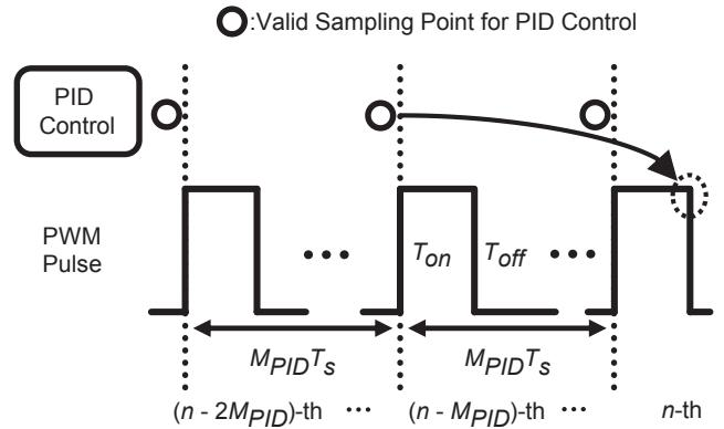
Fig. 2. Timing chart of PID control.
