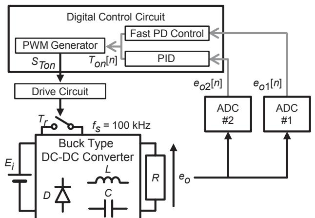
Fig. 1. Digitally controlled buck type dc-dc converter and scheme of digital control circuit.
