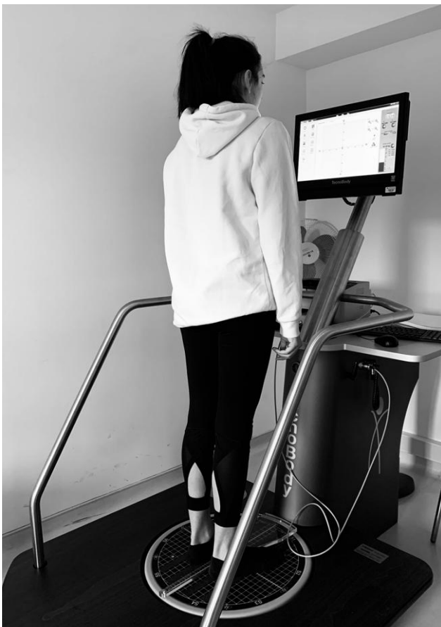
Figure 2. Assessment of static stability on the force platform via computerised stabilometer
