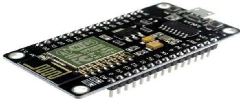
Figure11. ESP8266 NodeMCU WiFi Development Board
