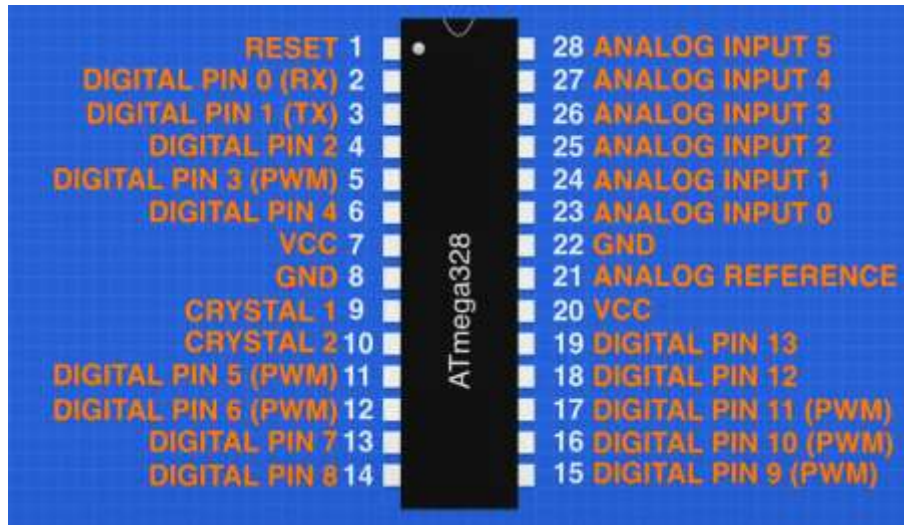
Figure 21. ATmega 328p pins in relation to Arduino
