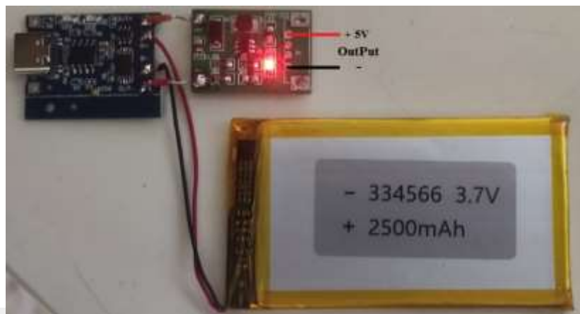
Figure 30. TP4065, SUB05V0600 and Battery
