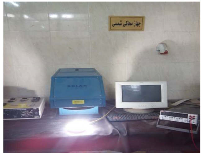
Fig. 2 The experimental setup of the solar simulation system.
