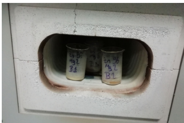
Fig. 2 The ash used for the synthesis of Zn_{0.98-x}Mg_{0.02}B_xO nanoparticles
