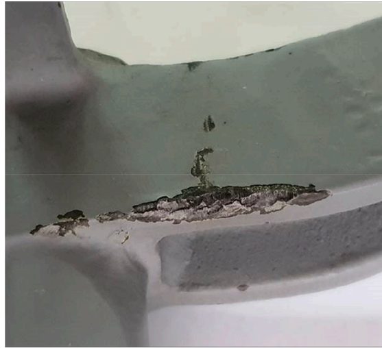
Fig. 4. Ratchet marks on the fractured surface.
