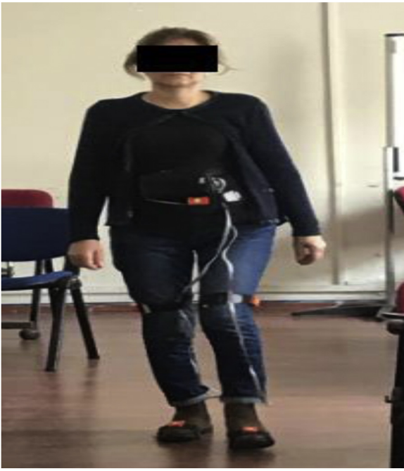
Fig. 6. Human subject with wearable motion sensors.
