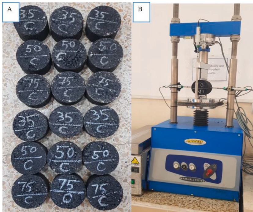
Fig. 4. (A) Condition samples (B) Indirect Tensile Strength (ITS) device.
