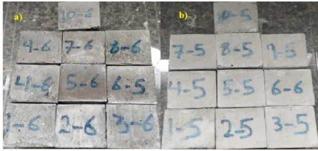
Fig. 5 The geopolymer (a) After exposure to magnesium sulfate solution 12 months (b) After exposure to sodium sulfate solution 12 months
