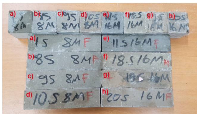
Fig. 19. Photo of the samples: a) Control-8M, b) CWA5-8M, c) CWA10-8 M, d) CWA15-8 M e) Control-16 M, f) CWA5-16 M, g) CWA10-16 M, and h) CWA15-16 M after 100 cycles.
