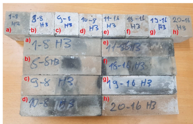
Fig. 12. Photo of the samples: a) Control-8M, b) CWA5-8M, c) CWA10-8 M, d) CWA15-8 M e) Control-16 M, f) CWA5-16 M, g) CWA10-16 M, and h) CWA15-16 M after 900 °C.
