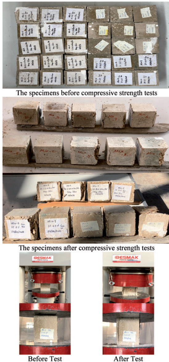
Figure 5. The specimens before and after compressive strength tests.
