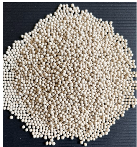
Fig. 3. Commercial synthetic 4A and 5A zeolite beads used in the tests.
