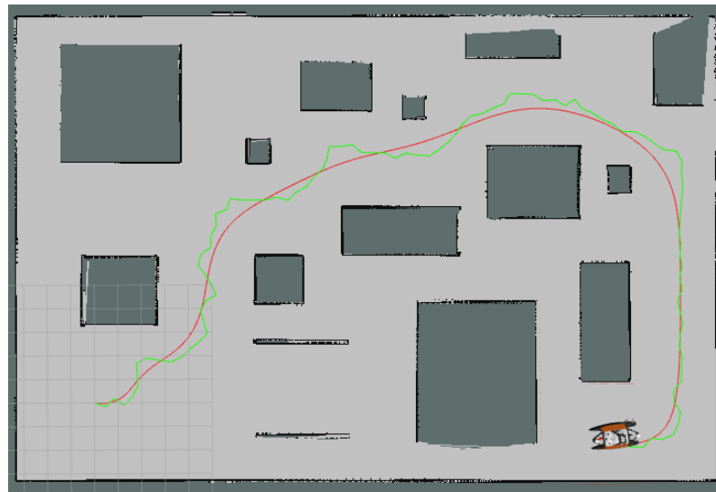
Figure 11. The Bézier Curve (red curve) and its control polygon (green polygon) for the second Map4 scenario.
