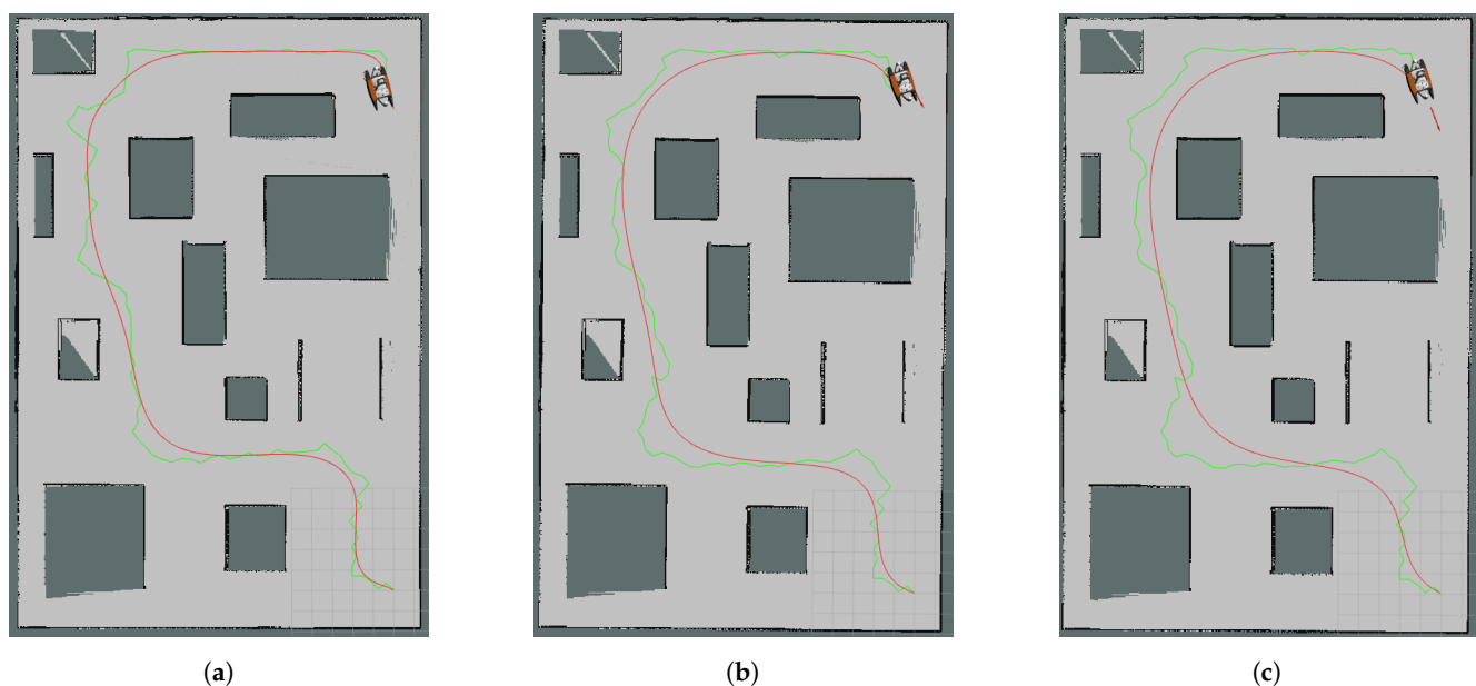
Figure 10. Curves (red curves) obtained for Map4 using the same control polygon which is also an RRT path (green polygon): (a) without control point reduction, (b) with 3 \times 1 mean filter control point reduction, (c) with 5 \times 1 mean filter control point reduction.
