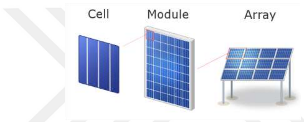
Figure 2. PV cell, module, and array structure.
