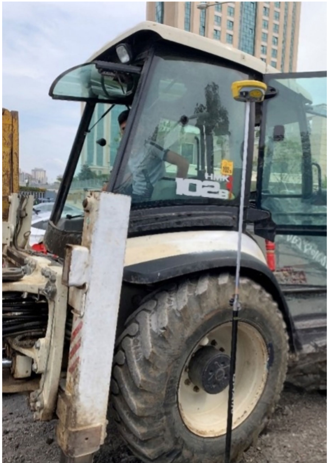
Fig. 6. Field validation procedure used to compare GIS-PIMS tracking outputs with survey-grade RTK-fixed GNSS reference measurements.
