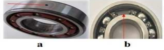
Fig.3 (a) Outer bearing, (b) Ball bearing faults
