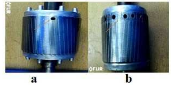
Fig.4 (a) One-broken rotor bar, (b) Five-broken rotor bars faults
