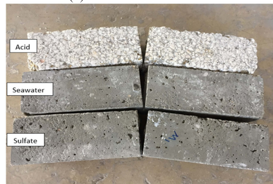
(d) Failure of the specimens under chemical solutions
