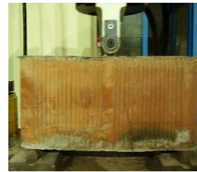
(c) Bending test on the brick specimen (ASTM C67)
