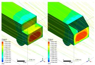
Figure 6. Pressure contours of truck models at 50 km/h
