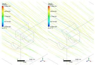
Figure 9. Velocity contours of truck models at 80 km/h
