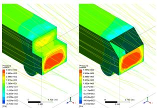
Figure 8. Pressure contours of truck models at 80 km/h
