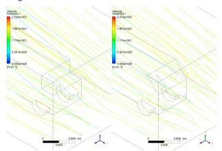
Figure 7. Velocity contours of truck models at 50 km/h
