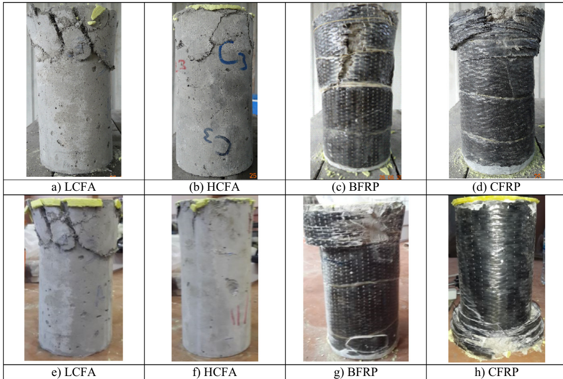
Fig. 8. Failure mode of SHCC specimens exposed to sulfate (a, b, c, d) and control (e, f, g, and h).
