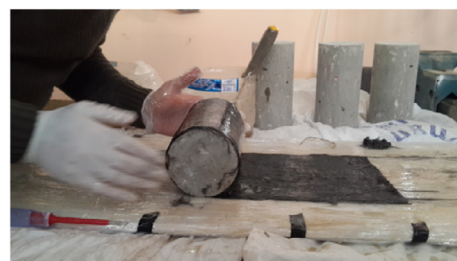
c) Application of FRP fabric
