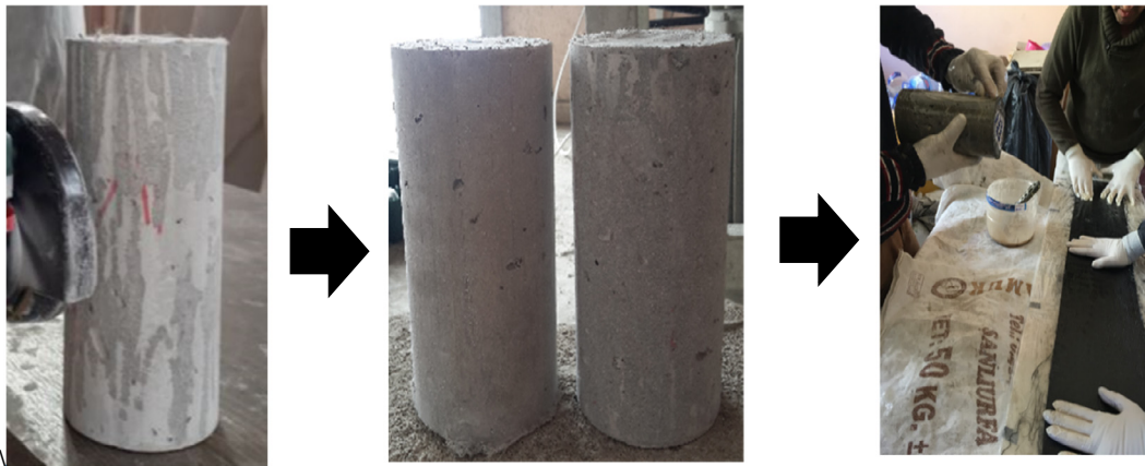
a) Concrete surface preparation
