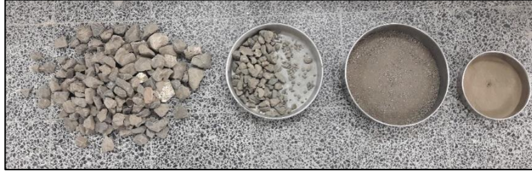
Şekil 6. Kirli balast (Fouled ballast)
