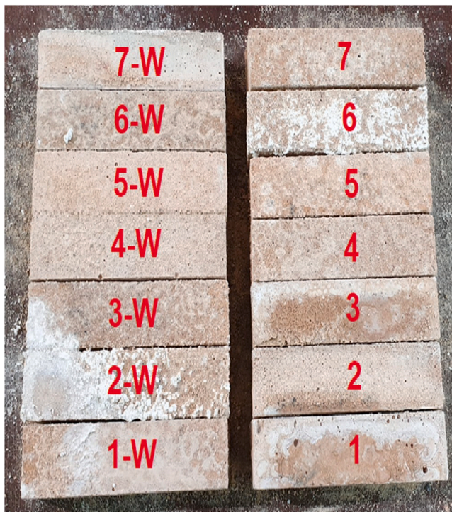
Fig. 9. Visual inspection after hydrochloric acid effect over 6 months.
