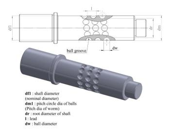
Fig. 4. Technical drawing of ball screw shaft
