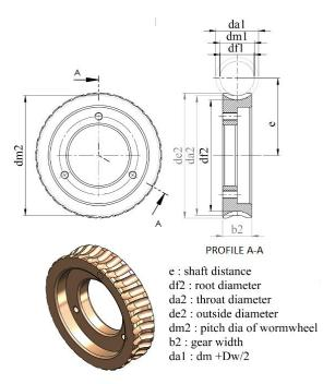
Fig. 5. Technical drawing of ball worm wheel
