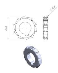
Fig. 6. Special semi-circular mouthed milling cutter
