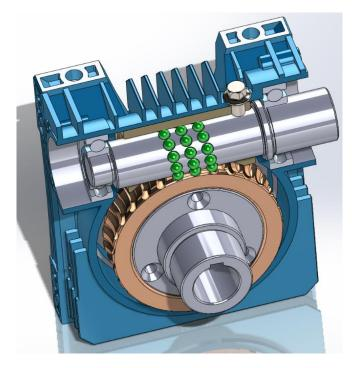
Fig. 8. Cross-section view of the assembled ball worm gear mechanism
