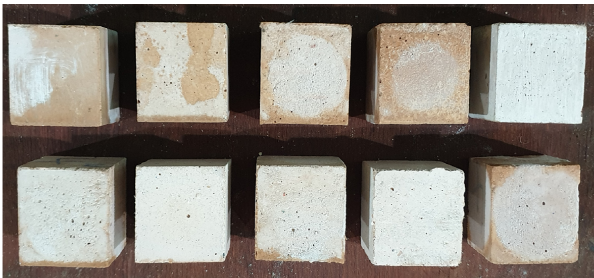
Fig. 32. Visual inspection after the freezing-thawing test.
