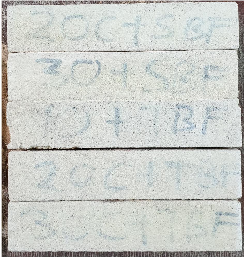
Fig. 23. Visual inspection after exposure to sulfuric acid over 3 months.
