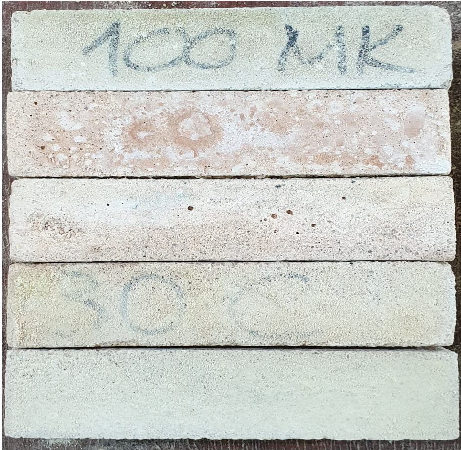
Fig. 22. Visual inspection after exposure to sulfuric acid over 3 months.
