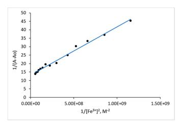
Figure 7. Benesi–Hildebrand plot for the 1:2 binding stoichiometry of azo 4c with Fe<sup>3+</sup>.
