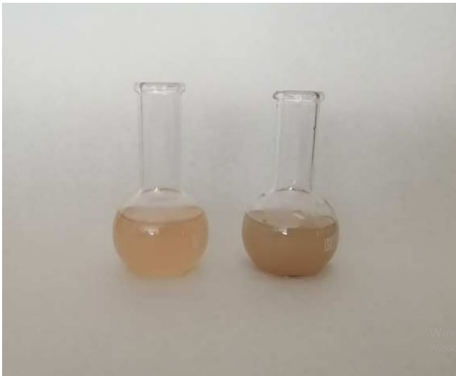
Figure 2. Ag NPs synthesized with 4 mM AgNO 3 in milk thistle seed extract.
