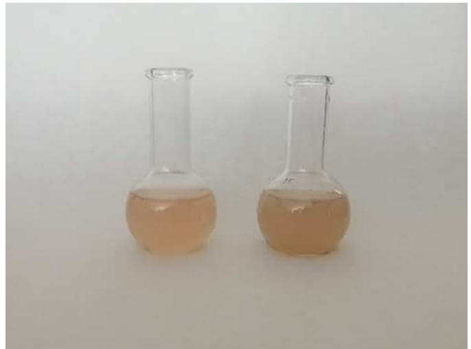
Figure 4. Ag NPs synthesized with 2 mM AgNO 3 in milk thistle seed extract.
