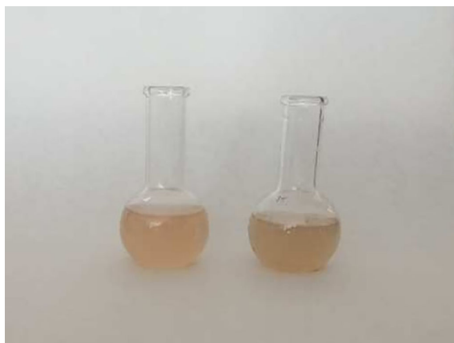
Figure 6. Ag NPs synthesized with 1 mM \text{AgNO}_3 in milk thistle seed extract.
