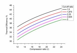
Fig. 1. The change in thermal efficiency according to different compression and cut off ratio in cases where ratio of specific heats  $(\gamma)$  is 1.2 constant
