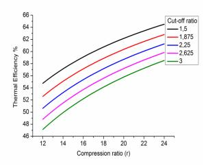
**Fig. 4.** The change in thermal efficiency according to different compression and cut off ratio in cases where ratio of specific heats (γ) is 1.35 constant
