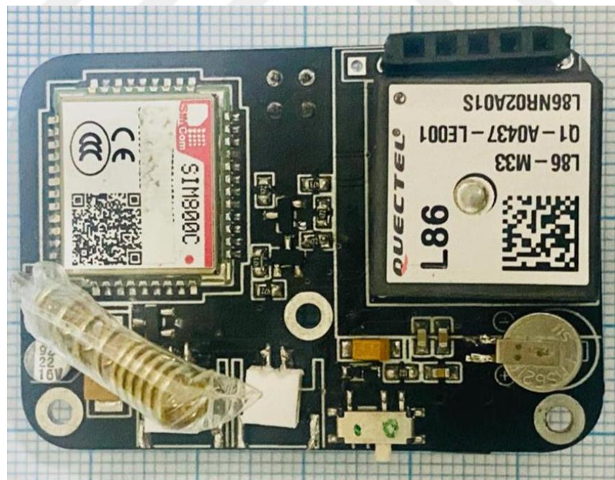
Figure 21. The Printed Circuit Board of the Designed Bracelet (Top Side).
