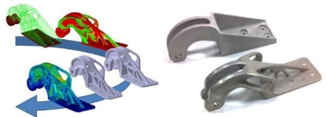
Figure 3: TO and AM Application of Airbus A320 Nacelle Hinge Bracket [18]
