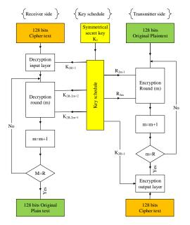
Figure 5 : Encryption/decryption structure
