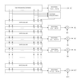
Figure 3. 128-bit Keys production
