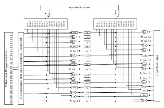
Figure 2. Digital Design of the Decryption Rounds Structure
