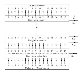
Figure 4: Encryption Structure
