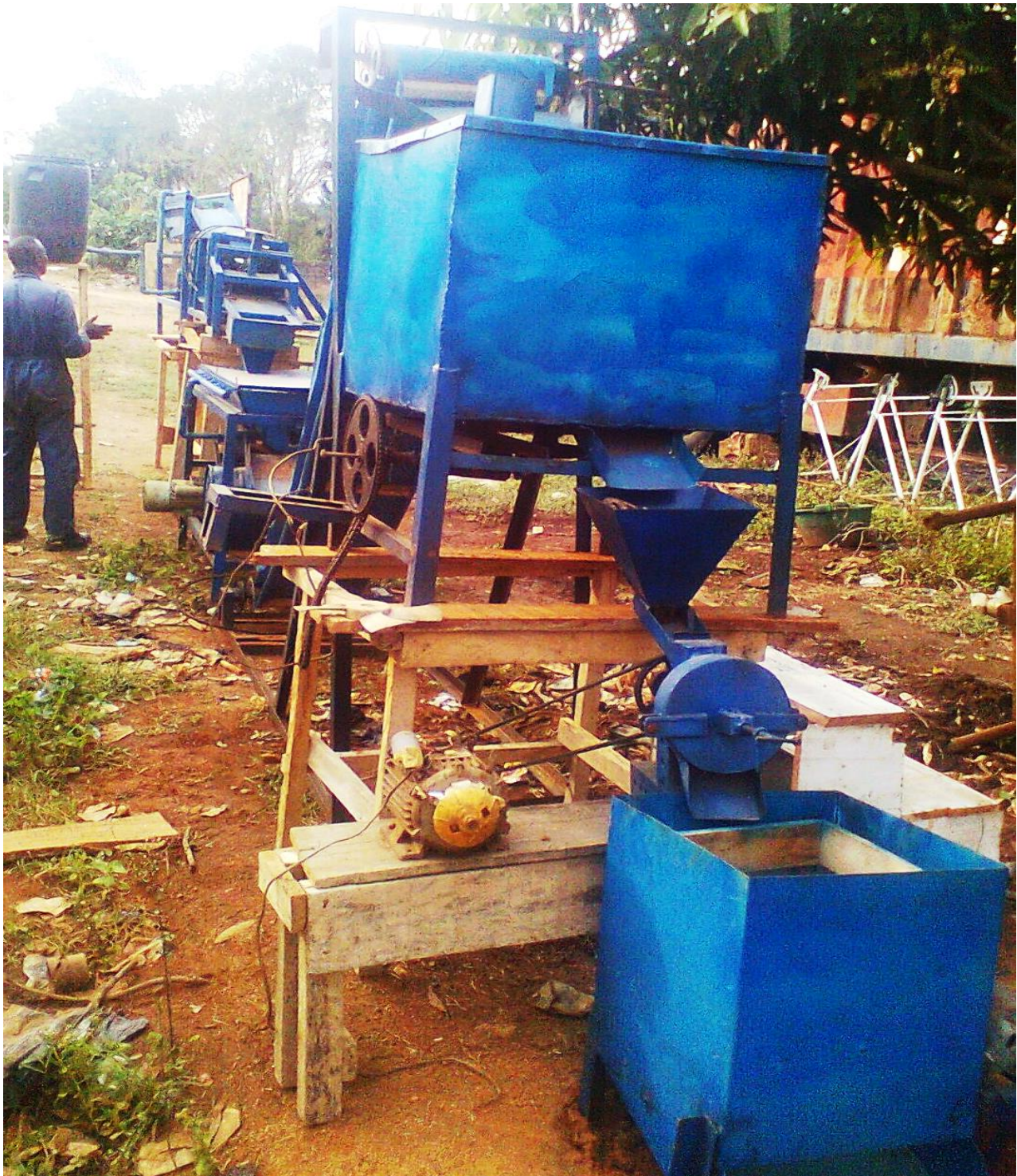
Fig. 3. Fabricated Poundo Yam Process Plant [20]
