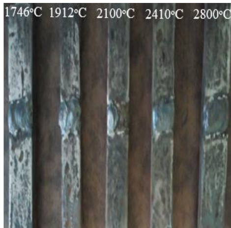
Fig. 2. Welded Samples showing Welding Temperatures
