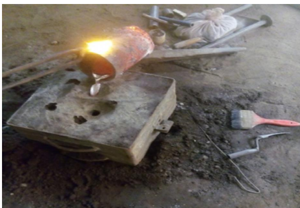
Fig. 2. Cast preparation by pouring the Al/SiC slurry from the crucible into the mould.
