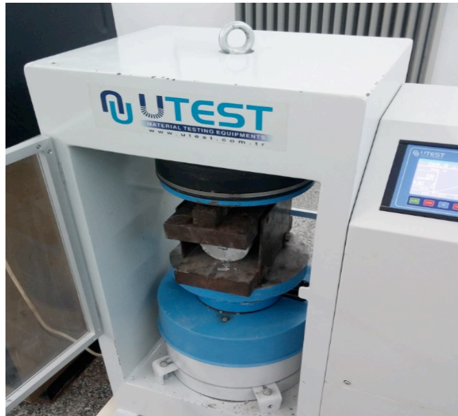
Fig. 2. Splitting tensile strength test
