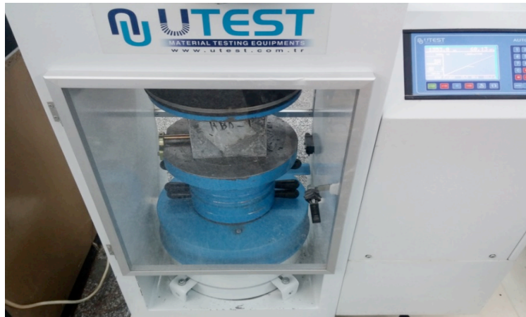
Fig. 1. Compressive strength test
