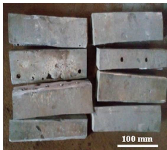
Fig. 1. Aluminum Al-4043 alloy ingots used in the study.
