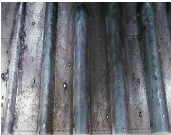
Fig 1. Workpiece welded with 50A Current
