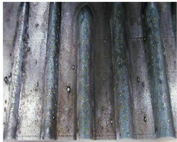
Fig 3. Workpiece welded with 150A Current
