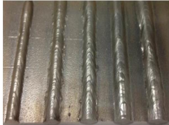
Fig 2. Workpiece welded with 100A Current
