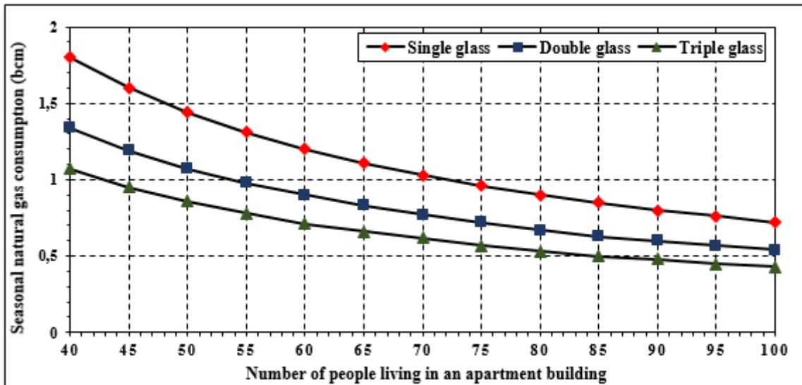
Fig. 5. Seasonal natural gas consumption in Kocaeli for GAP=35% and I=1.0 ACH versus number of people living in an apartment building.
