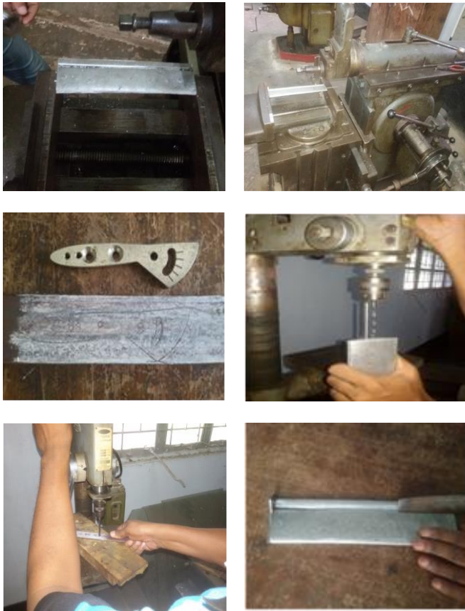
Fig. 3. Preparation of an aluminum NACA 0015 blade.
