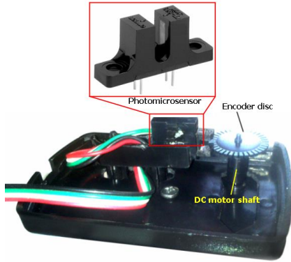
Fig. 5. Encoder unit including an encoder disc and photomicrosensor
