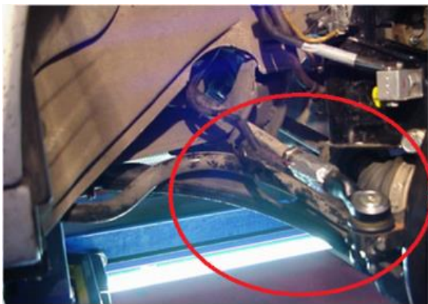
Fig. 5. Steering wheel tie rod with strain-gauge assembled on the vehicle
