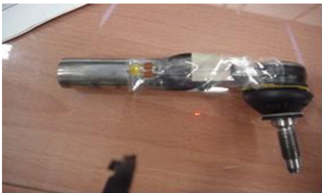
Fig. 4. Steering wheel tie rod with strain-gauge applied
