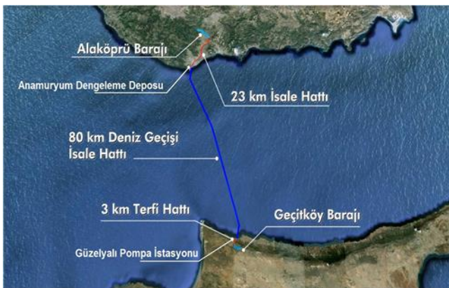
Fig. 2. Plan of transmission line between Turkey and TRNC [6]
