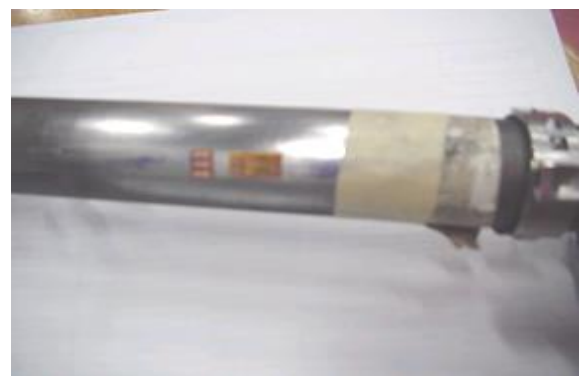
Fig. 3. Strain-gauge mounted on driving shaft in laboratory
