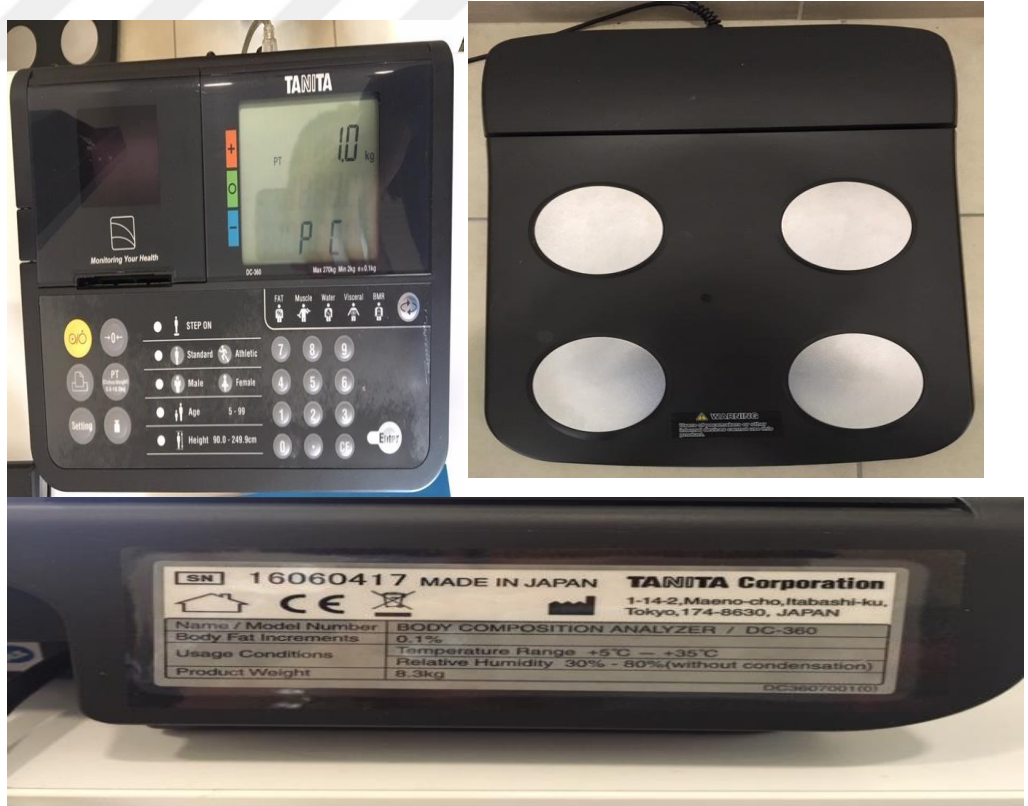
Şekil 3.1.Tanita Corporation (Model: Body Composition Analyzer/ DC-360).
