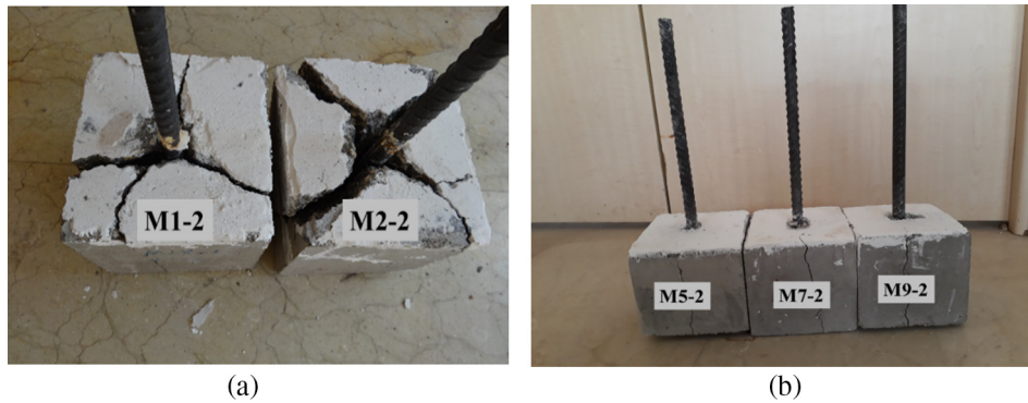
Fig. 9. The fracture patterns of SCGCs: (a) without SF and (b) with SF.
