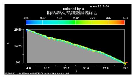
Figure 10. Change of horizontal flow rate on Salı Pazarı Yokuşu model section
