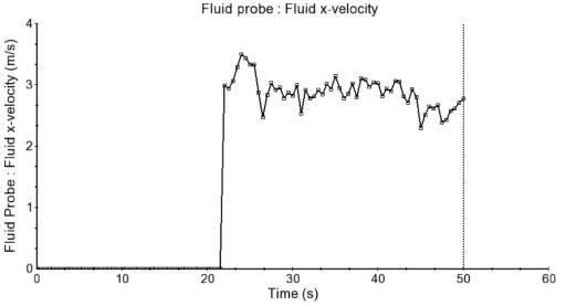
Figure 6. Horizontal flow velocity values at fluid probe of the Enli Yokusu model (m/s)
