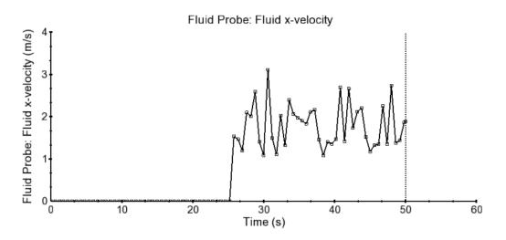
Figure 9. Horizontal flow velocity values at fluid probe of the Salı Pazarı Yokuşu model (m/s)
