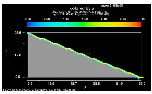
Figure 7. Change of horizontal flow rate on the Enli Yokuşu model section
