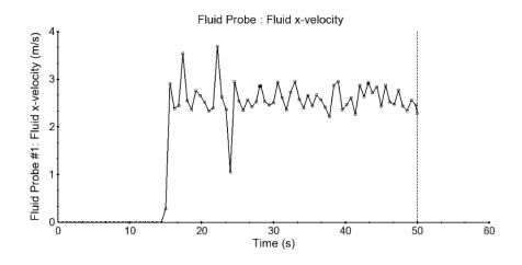
Figure 3. Horizontal flow velocity values at fluid probe of the standard model (m/s)
