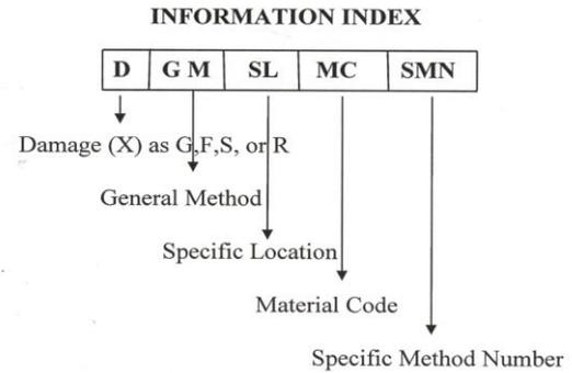
**Fig. 3** Specification of repair methods
