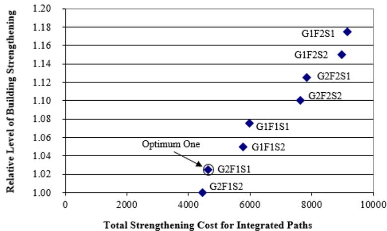
Fig. 10 Integrated path evaluation – cost versus strengthening level
