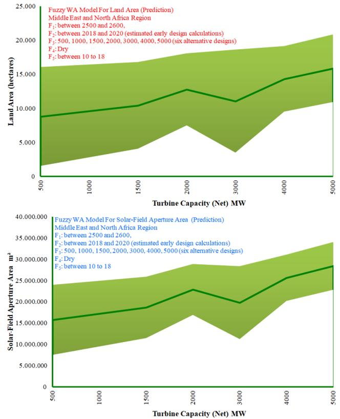
**Fig. 7.** FWA land area APE per project, FOWA land area APE per project, FWA solar field aperture area APE per project, FOWA solar field aperture area APE per project, FWA land area predictions, FWA solar field aperture area predictions (open ESM and FuzzME model files) \*Note: from top to bottom.
