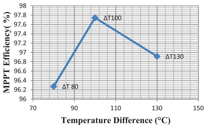
**FIGURE 17** The efficiency of PD-MPPT algorithm under various  $\Delta T$  for three parallel connected TEG [Colour figure can be viewed at [wileyonlinelibrary.com](http://wileyonlinelibrary.com)]
