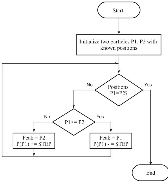
FIGURE 12 The flowchart of PD-MPPT algorithm
