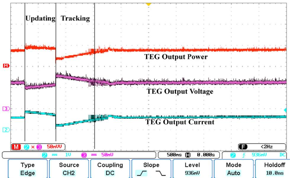
**FIGURE 14** The output power, current and voltage of three series TEP1-142T300 with STM32F429 microcontroller [Colour figure can be viewed at wileyonlinelibrary.com]
