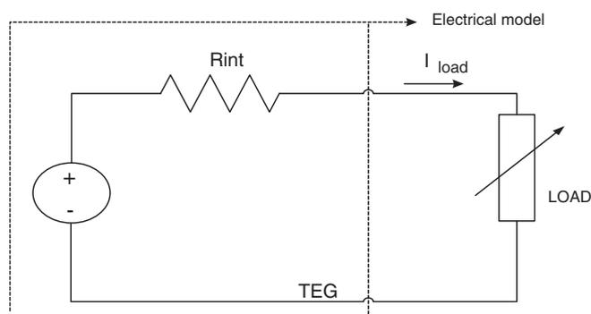
FIGURE 1 Electrical model of a thermoelectric generator
