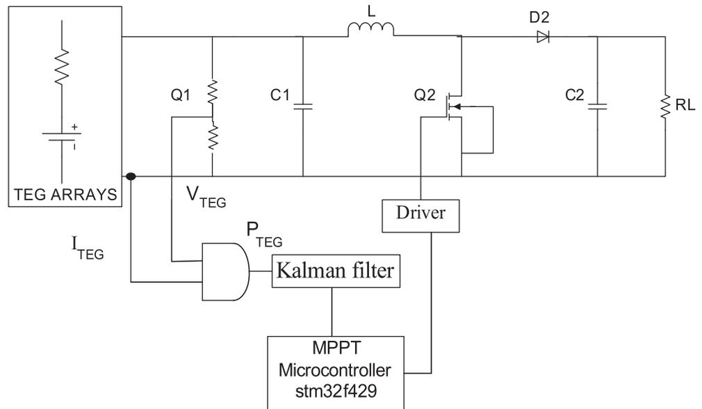
Figure 9 reveals the constructed diagram of the proposed power generation system.
