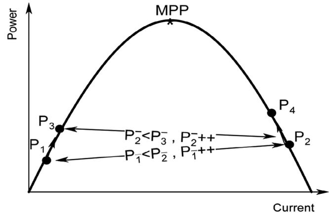
FIGURE 11 The mechanism of the PD-MPPT algorithm
