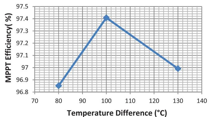
**FIGURE 16** The efficiency of PD-MPPT algorithm under three different  $\Delta T$  for three series connected TEGs [Colour figure can be viewed at wileyonlinelibrary.com]
