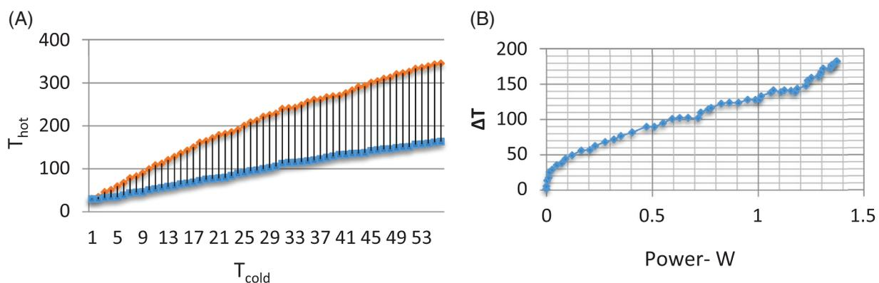
**FIGURE 7** (A) The increment of temperature difference on TEG Surfaces and (B) the relation between TEG output power and temperature difference  $\Delta T$  [Colour figure can be viewed at wileyonlinelibrary.com]
