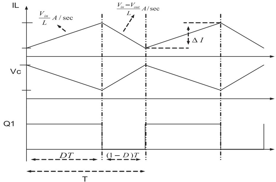
**FIGURE 9** Continuous conduction mode of the boost converter
