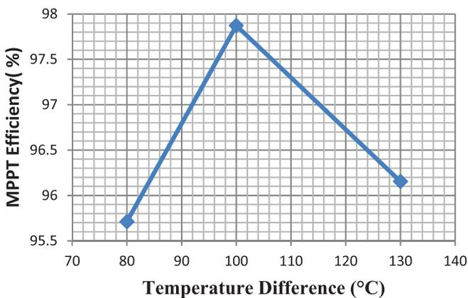
**FIGURE 15** The efficiency of PD-MPPT algorithm under various  $\Delta T$  for single TEG [Colour figure can be viewed at wileyonlinelibrary.com]
