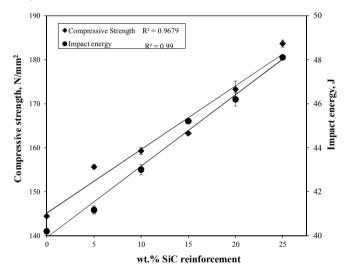
Fig. 8. An increase in compressive strength and impact energy of composite with increasing wt.% SiC reinforcement.
