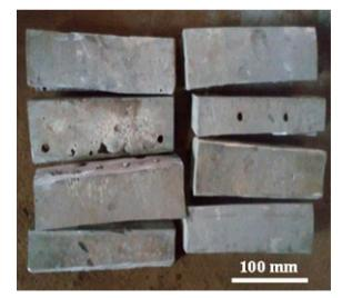
Fig. 1. Aluminum Al-4043 alloy ingots used in the study.
