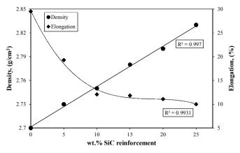
Fig. 6. An increase in density and decrease in elongation of the composites with increasing wt.% SiC reinforcement.
