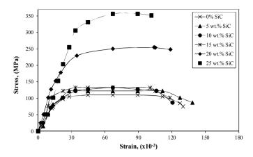
Fig. 4. The stress-strain curves for the Al-4043/SiC composites with variation in wt.% reinforcement.
