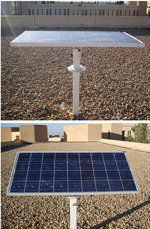
FIGURE 2 Manually solar tracking model with panel of model KC120-1 6 [Colour figure can be viewed at wileyonlinelibrary.com]
