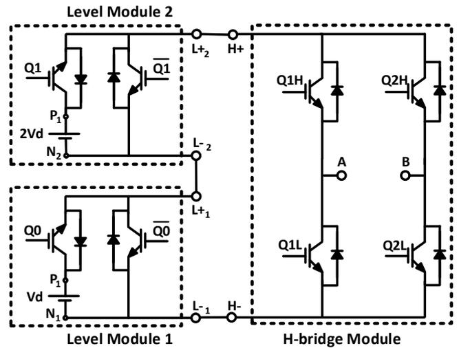
**Fig. 2.** The principle scheme for 7-level half-bridge cascaded inverter
