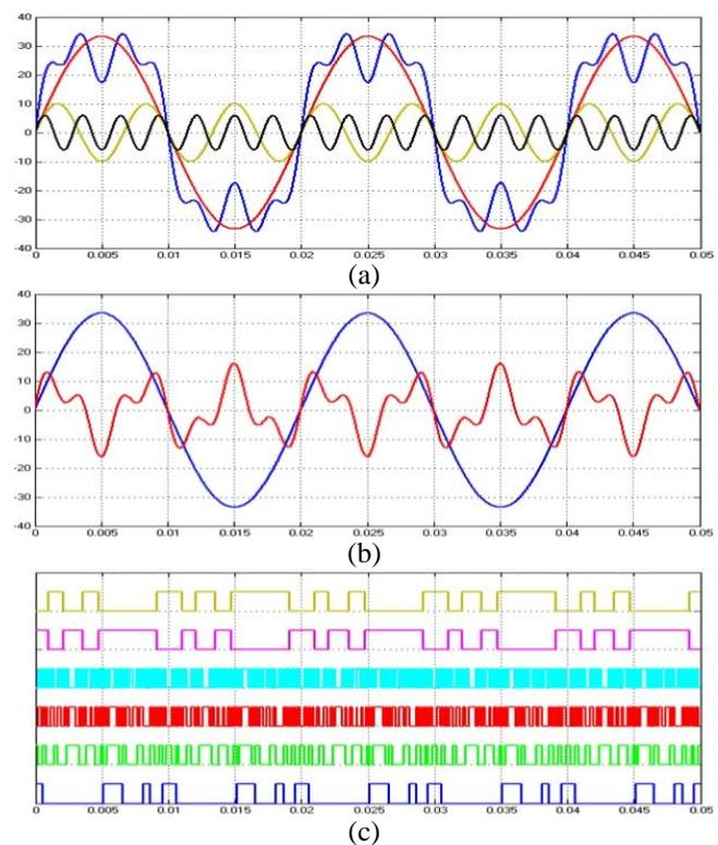
**Fig. 8.** The simulation results obtained from 31-level inverter based parallel active power filter, a) grid current with a THD value of 34.99% and harmonic components before filtering, b) grid current and filter current, c) switching signals
