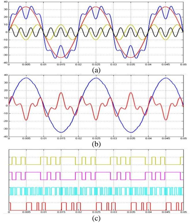
**Fig. 7.** The simulation results obtained from 7-level inverter based parallel active power filter, a) grid current with a THD value of 34.99% and harmonic components before filtering, b) grid current and filter current, c) switching signals
