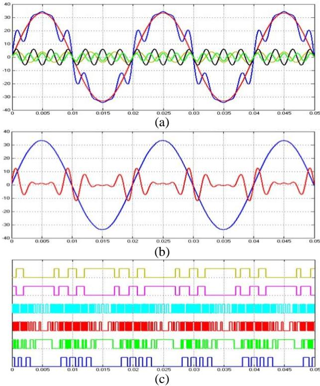
**Fig. 6.** The simulation results obtained from 31-level inverter based parallel active power filter, a) grid current with a THD value of 23.43% and harmonic components before filtering, b) grid current and filter current, c) switching signals
