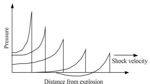
Fig. 1. Blast wave propagation (Abaqus 6.10)
